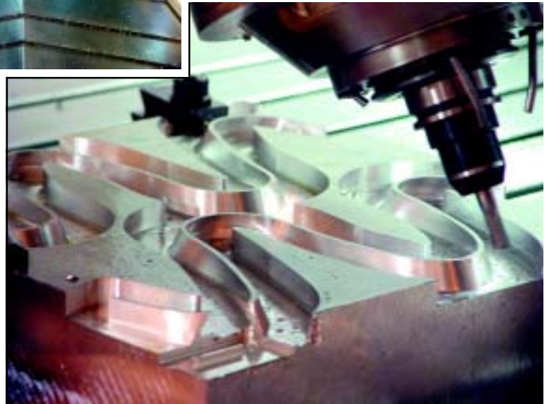
Thin wall and deep pocket sections of aerospace parts are handled easily, with speed and accuracy unavailable in previous generation machines.
